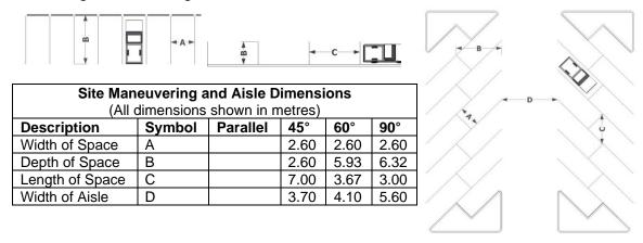
Parking space length may be reduced to 4.57m for isolated spaces (caused by column placement, etc.) up to 5% of the number of required spaces. Such spaces must be clearly marked "small auto only" on the pavement or wall facing. In lots exceeding 100 spaces in number, up to 20% of the spaces may be reduced to 4.57m in width provided those spaces are provided in groups of at least 20 spaces
