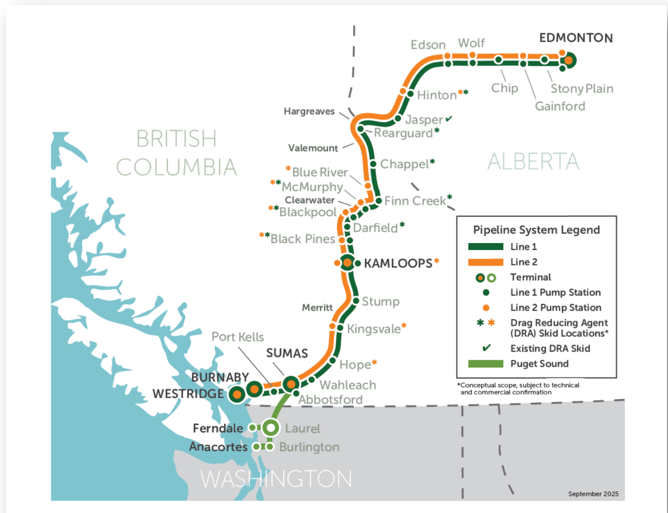
Figure 1: DRA Unit Pump Station Locations
